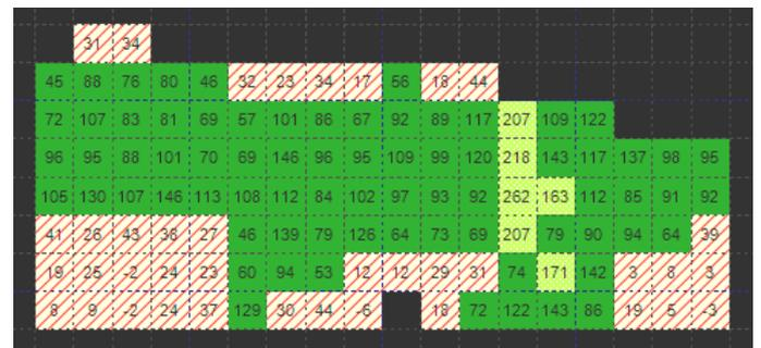
2D plot showing graphically the sprayed result divided in three classes of thickness:
