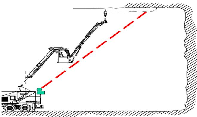
Movements during shotcrete spraying is monitored and corrections are applied if needed. The system is handled by the shotcrete robot operator.
