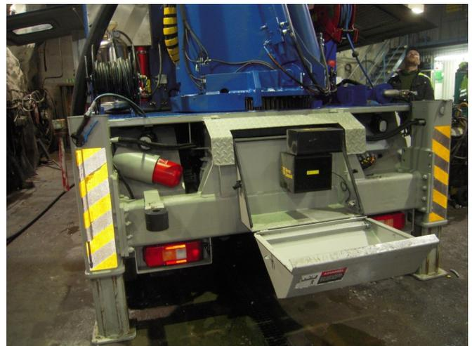
Placement of Bever 3D Profiler, automatic docking under a protective hood for easy cleaning
