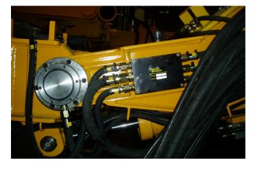
Mechanical, hydraulic and electric components on the jumbo are best quality and well protected. Sensors have robust mechanical enclosures, and cables on the booms are protected in hydraulic hoses.
