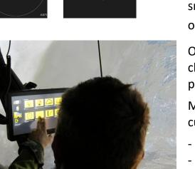
Round drilling and blast pattern adjusted to expanding tunnel cross-section area. Face view and top view can be displayed. From the face view, we display actual collar position and look-out. Top view shows planned and actual drilling depth. The depth hole can be accurate controlled to obtain a preprogrammed bottom face. Reduced scaling, smooth blasting and reduced vibration can be obtained
