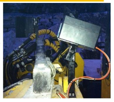
A series of pictures are taken in different angles when the operator pushes the start button on the control screen.
